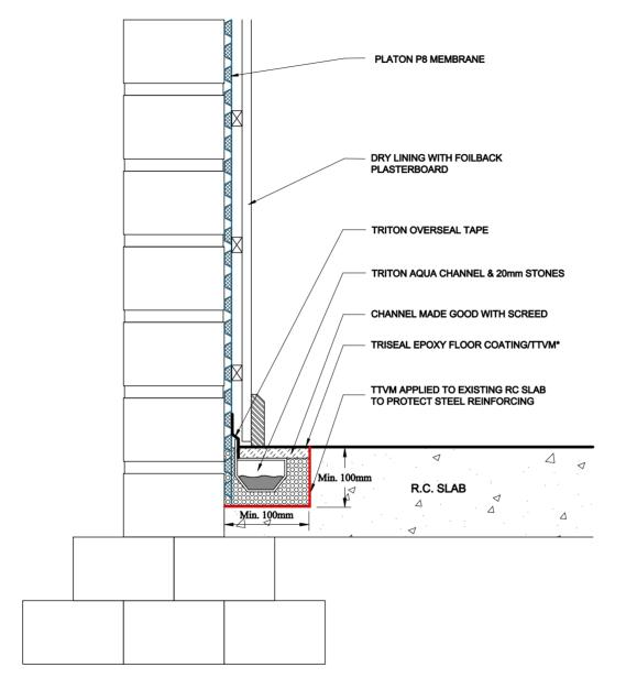
\* When using TTVM a suitable screed or protective floor layer is required!
