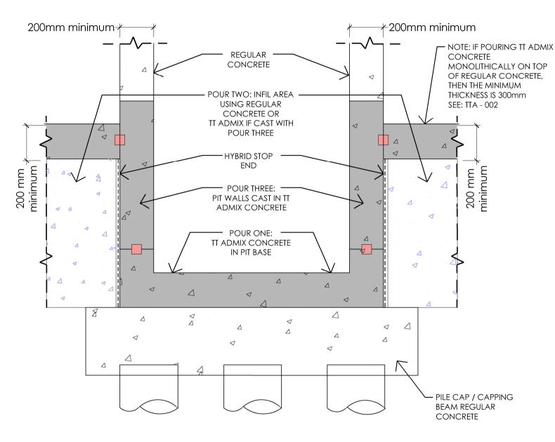
TT WATERSTOP BONDED WITH IT SWELLMASTIC (INSTALLED INTO A PRE-FORMED REBATE)
