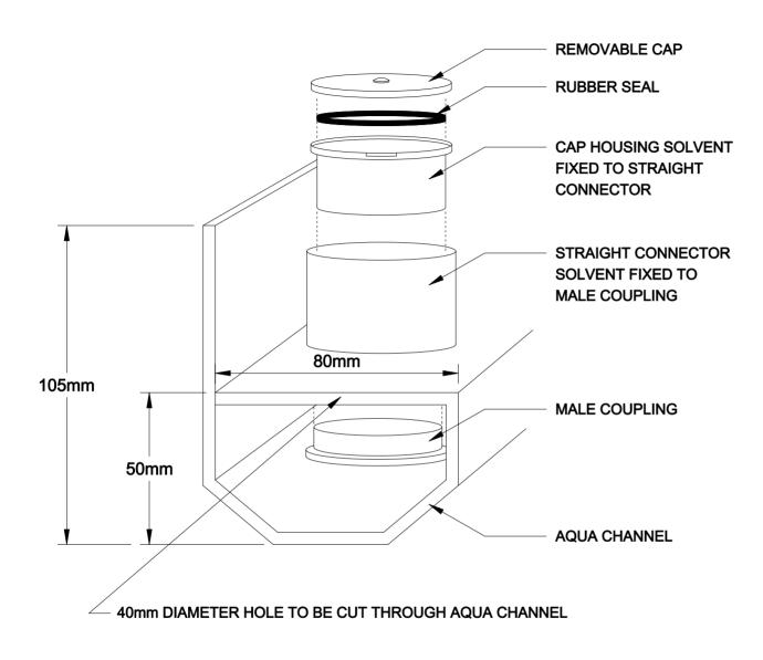
RODDING EYE CAN BE EXTENDED TO SUIT USING STANDARD 40mm PIPE PLUS CONNECTORS
