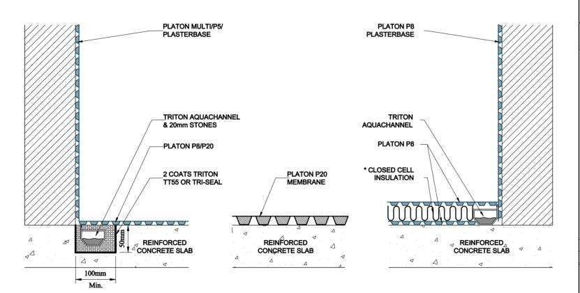
\* INSULATION MUST BE SUITABLE FOR USE ON DAMP SIDE OF MEMBRANE AND MUST HAVE SUITABLE POINT LOADING STRENGTH
