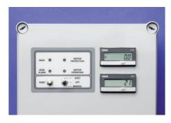
This single pump control unit contains an integral high level alarm, both audible and visual, and visual counters which record the number of pump activations and length of run time.
