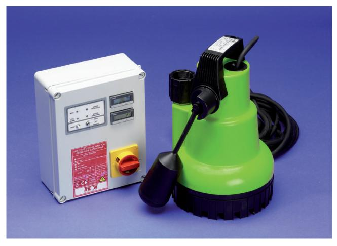
The unit controls the activation of the pump by way of a float mechanism which is located in the sump chamber. The high level float mechanism is set at a level just higher than that of the pump. When installed, the panel will enable contractors and pump service engineers to monitor the pump's activity during the period between service visits and will indicate the volume of water entering the installed cavity drain system.
