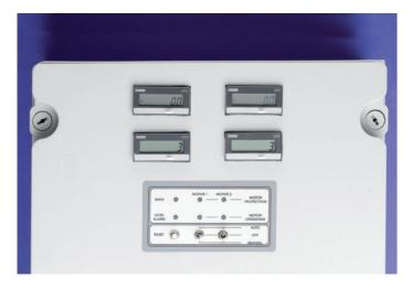
The Dual Assist Control Panel is provided with integral high level alarm and monitoring capabilities to monitor the number of activations and length of run times for each of the two main pumps. Both pumps and the high level alarm are operated by the control panel via float switches located in the sump.
