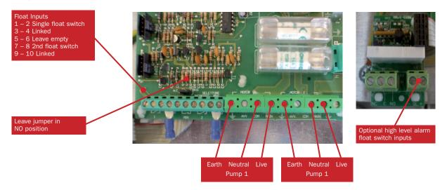
The panel is designed to control two pumps with either a single float or dual floats. An optional high level alarm float may be installed, set above the highest pump float, to warn of excessive water level.
