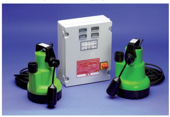
Where two pumps are installed in a single sump then the Dual Assist Control Panel will activate both pumps alternately and also in times of high water ingress, will activate both pumps to operate simultaneously.
