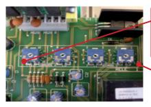
Motor current overload trimming potentiometer Set values to motor rated current plus 10% for each pump
