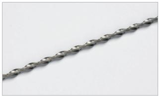
Stainless steel Tribar Rods are designed to stabilise existing masonry and are used in general crack stitching repairs, to reinforce masonry above failed lintels, as a method of overpinning to reduce the underpinning load and to re-tie solid or cavity masonry panels. Typical applications will be in buildings with shallow foundations or which are subject to movement, masonry arches and bridge repairs.
