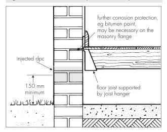
13.4 If the timbers are sound, the existing floor may be retained provided the injected dpc is formed below the timber joists and/or wall plate (see Figure 4).
