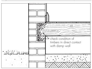
13.3 If damage is limited to the joist ends, the floors may be re-formed, using sleeper walls or joist-hangers, to isolate the timbers from the damp wall (see Figure 3).
