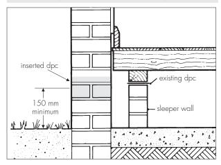
13.2 Where a suspended timber floor is supported on joists and/or a wall plate bearing on or embedded in the wall, there is a possibility of decay, particularly where concealed timbers are in contact with the damp wall. The condition of these timbers should be ascertained and remedial action taken if necessary (see Figure 2).
