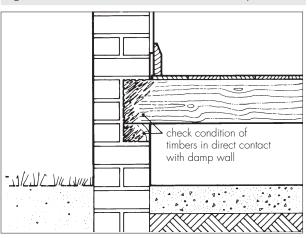
13.3 If damage is limited to the joist ends, the floors may be re-formed, using sleeper walls or joist-hangers, to isolate the timbers from the damp wall (see Figure 3).
