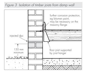
13.4 If the timbers are sound, the existing floor may be retained provided the injected dpc is formed below the timber joists and/or wall plate (see Figure 4).
