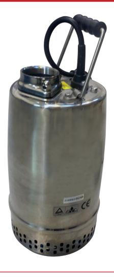
The RS55 is a highly reliable waste water pump offering a stainless steel shaft, outer and motor casings. The twin mechanical seals provide a long service life. The pump can be supplied with a conventional ball type 'MAC 3' float, fixed magnetic canister 'AGMA' float, or without a float for manual operation, making this unit highly flexible. The top outlet allows installation in narrow sumps. Supplied free standing for quick installation.
